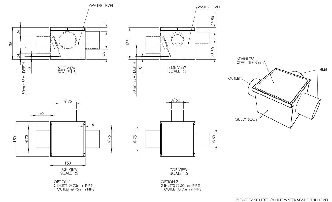
PLEASE TAKE NOTE ON THE WATER SEAL DEPTH LEVEL FOR BOTH INLET PIPES (75 & 50mm INLET PIPE)
